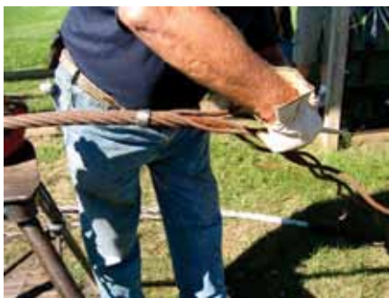
Cutting out core at marriage point.
